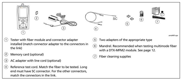
Figure 10. Equipment for Testing in Loopback Mode (Method B)
