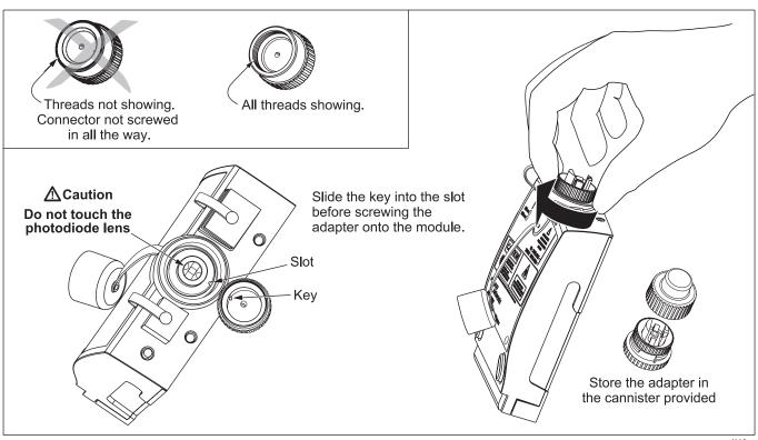
Figure 4. Installing the Connector Adapter
