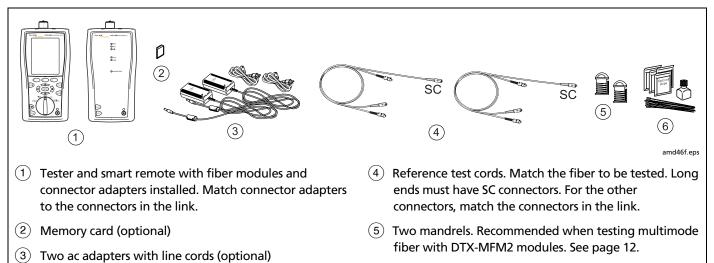
Figure 7. Equipment for Testing in Smart Remote Mode (Method B)
