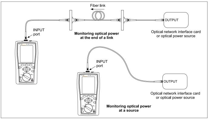
Figure 19. Connections for Monitoring Optical Power
