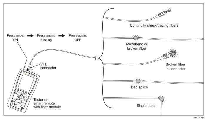
Figure 17. Using the Visual Fault Locator
